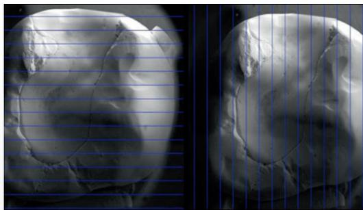
**Fig. 4.** Horizontal and vertical test lines, superimposed on a SEM-picture, to calculate the length of the discrepancies (original magnification 16 x).
