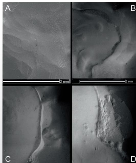
**Fig. 2.** Smooth margin (A), excess composite material (B), gap (C), chipping (D) (original magnification 16 x).
