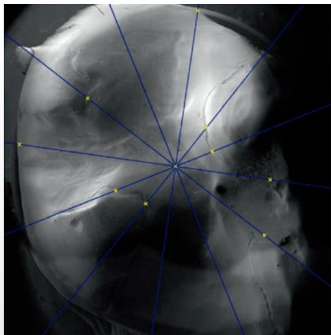
**Fig. 3.** 2D isotropic test lines, superimposed on a SEM-picture, to calculate the width of the discrepancies (original magnification 16 x).
